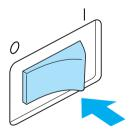
▶ The buzzer beeps once and the LCD screen comes on.
